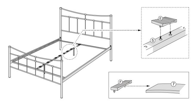
**Step 6**: Slide the Slats (7) into hardware part (E) on the Mid Support (5) then push the ends into the Side Supports (3) firmly, insert hardware part (G) to the frame posts.
