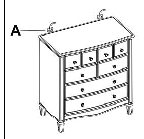
Step1. Drill a hole into the wall and press the wall plug (E) into the hole. Use the long screw(C) to securely attach the bracket (A) to the wall by using allen key (F).
