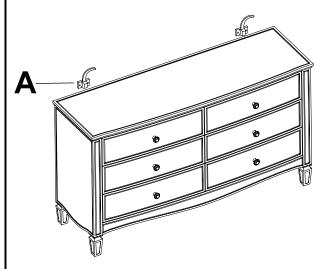
Step1. Drill a hole into the wall and press the wall plug (E) into the hole. Use the long screw(C) to securely attach the bracket (A) to the wall by using allen key (F).
