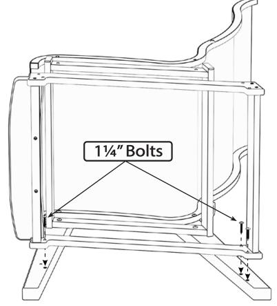
Attach Footrest Assembly to Leg Assembly using (3) 11/4" Bolts.
