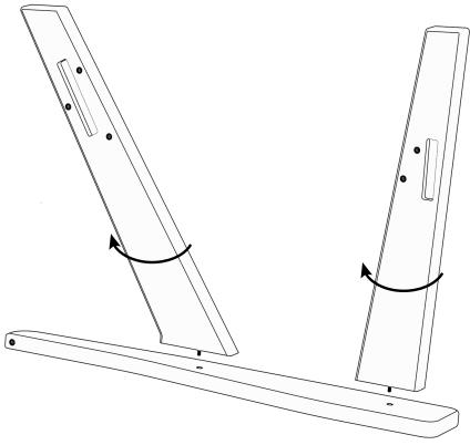
Thread the front and back leg in to the inserts as shown above. Repeat on the opposite arm and legs.
