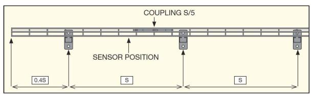
Note: The maximum deflection of 1/100 is always reached for a lesser load than that of the safety load. (The breaking point divided by a safety co-efficient of 1.7). CEI/61537
