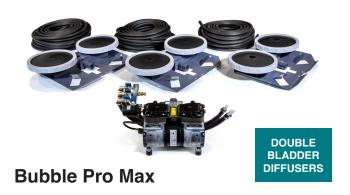
The Bubble Pro Max comes complete with three diffusers; three lengths of 100-foot by 3/8" Quick Sink weighted tubing; a 1/2-hp, rocking-piston compressor; a valved air outlet assembly with individual controls for each hose and a pressure relief valve; and all required fittings and clamps. Designed for easy installation, the Bubble Pro comes with a two-year warranty. Also available for 230-volt power.
