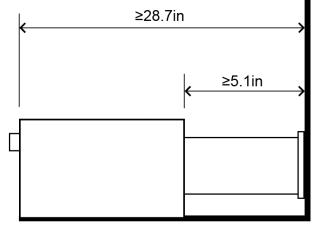
Follow the UP icon, the vents must be installed as shown.
