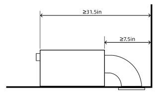
Make sure the vent location has free airflow and is free of direct obstruction within 8 inches.
