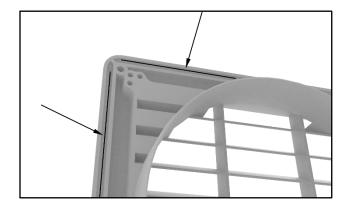
• On the inside, place the trim over the opening. Use self-tapping screws to secure the inside vent piece to the outside vent piece.
