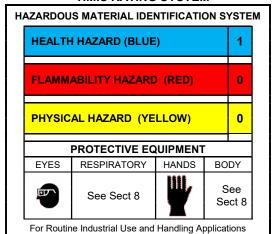
Hazard Scale: 0 = Minimal 1 = Slight 2 = Moderate 3 = Serious 4 = Severe \* = Chronic hazard
