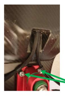
Remove these 2 truck mounting nuts on front truck (3/8" socket on nut and 1/8" allen on truck bolt on top side). Then slide the cable clamp off the protruding bolt and remove the old cables from inside. Now put the new LED cables into the cable clamps, slide back onto bolt and tighten nut. Note orientation of cable clamps in pic.
