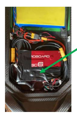
Reapply electrical tape as shown. Be sure cables have a bit of slack before putting the tape back in place on top of them. The purpose of this tape is to make sure the cable connectors don't vibrate loose during riding. Also make sure the cables are not routed on top of any of the protruding bumps or screws on the MESC LID. They should only be lying on the flat surfaces of the LID.
