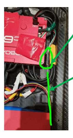
Note if you received a new NRF51 BT module it can be velcroed to the side of the MESC6 Case as shown with antenna oriented as shown by green line
