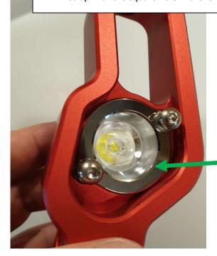
**FIRST:** Insert the Reflector/Lens assembly into the front truck opening using the usual mounting screws and split lock washers (be careful not to bump the lens against the truck hole so it doesn't lose its orientation from last step)
