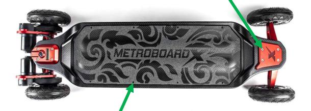
Remove the 8 lid screws (2.5 mm allen) and remove the lid from the deck
