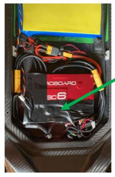
Carefully peel back the electrical tape covering the MESC (and save for reassembly later)
