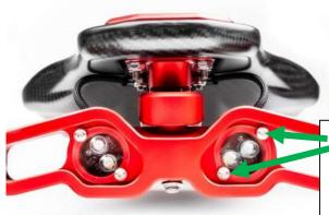
Remove existing lights by removing the two long screws that go through the lens in the front hanger. Use a 2.5 mm allen. Be careful not to lose the split lock washer attached to these screws
