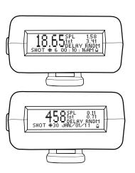
START button. After the beep, fire shots; the timer will display the rounds per minute based on the number of shots and the time between the first shot and the last. Shots recorded more than 199.99 seconds after the start beep will render readings invalid until START is pressed again. The normal shot dead time setting is overridden when in RPM mode and set to a fixed value of 0.032 seconds. This allows the PocketPro II to detect shots at rates of up to 1800 RPM.
