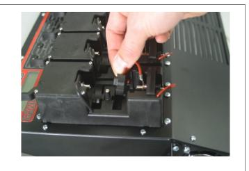
then removing, rotating and inserting the cell rotors into the holder so that the proper cell diameter and length is selected.
