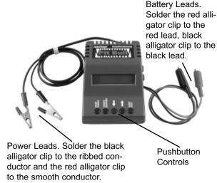
After assembling the cable, plug it in to the back of the Pit Bull, and connect it to your DC power supply, being careful to observe the proper polarities. As soon as you apply power, the display will illuminate and display the sign-on message. After this, it will display the message, PIT-BULL Ready!
