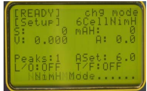
Figure 13: Typical status screen showing the mode display in the upper right hand corner
