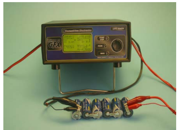
Figure 6: Typical Nixx Sense and Power Lead Connections
