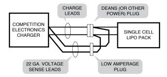
Note that the sense leads are connected through a dedicated connector to the other side of the power connector. This way, error due to any significant source of voltage drop across the power connector is eliminated.
