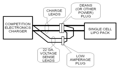
Note that the sense leads are connected through a dedicated connector to the *other side* of the power connector. This way, error due to any significant source of voltage drop across the power connector is eliminated.
