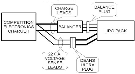
Here, the pack has a Dean's connector for the main power connections and a special pin and socket connector for the balance function.
