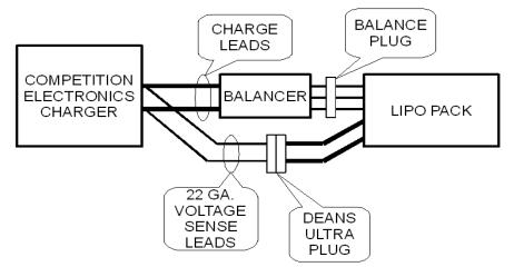
Here, the pack has a Dean's connector for the main power connections and a special pin and socket connector for the balance function.
