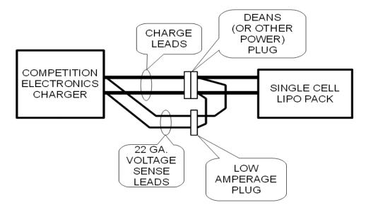
Note that the sense leads are connected through a dedicated connector to the *other side* of the power connector. This way, error due to any significant source of voltage drop across the power connector is eliminated.
