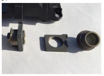
NOTE: Late model Cup shifters use 997 cradles, which Porsche Motorsport modified by sanding out the inner cradle barrels to fit the 996 Cup bushings. Depending on how much material they removed, you may need to lightly and evenly sand out the inside of the cradle barrels a bit more to provide sufficient clearance to fit the SHIFT-RIGHT bushings.
