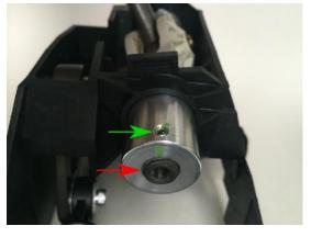
4. Confirm there is no end play by rotating the shifter side to side, fore and aft, and also make sure there is no binding. Operation in all directions should be smooth. If not, loosen the large set screw until smooth operation is achieved.
