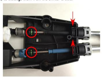
3. Unscrew the 4x 10mm nuts to remove the shifter assembly from the car, and transfer the shifter onto a workbench.
