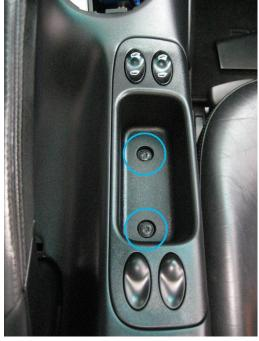
Fastener #3: Remove coin holder from rear storage bin (insert small pry bar in slot at coin holder base and pry upwards) to access fastener #3 (circled in GREEN).
