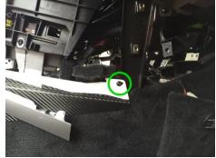
5. Remove the storage cubby bin via the 2 screws (circled in RED) and remove the screw (circled in GREEN). Pop the E-brake cover off by lifting from the rear and tilting it forward until fully released from the console, then remove the screw (circled in BLUE). Remove rubber mat from the rear storage bin to access and remove the 4 remaining screws (circled in YELLOW). Unplug the center console's wiring harness below the center stack prior to console removal.
