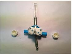
5. Push the white pin outward from the inside of the shifter cradle to release the shifter yoke. Remove the cable end by pressing the black pin out from the back of the yoke.
