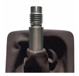
2. Set desired height and orient the shift pattern (if applicable): First, slide the base onto the shift lever and snug one of the bottom set screws. Now, using the wave washer betwn the base and knob, fully tighten down the shift knob. Loosen the set screw and rotate the shift knob to the correct orientation and desired height, and fully tighten the set screw.
