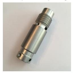
3. With the bottom set screw fully tightened, unscrew the knob halfway to fasten the top set screw that is directly above the bottom set screw. Then, fully tighten down the shift knob onto the base. Ensure that the shift pattern is clocked properly - if not, return to the steps above. Finally, rotate the shift boot to the correct orientation and reinstall into the center console.
