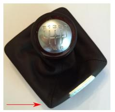
2. **Separate the shift boot from the knob:** To separate the knob from the boot, twist the boot until you're able to release the shift knob fingers from the boot collar. Once separated, remove the plastic inner and outer collars from the boot as you will not be re-using these with the new shift knob.
