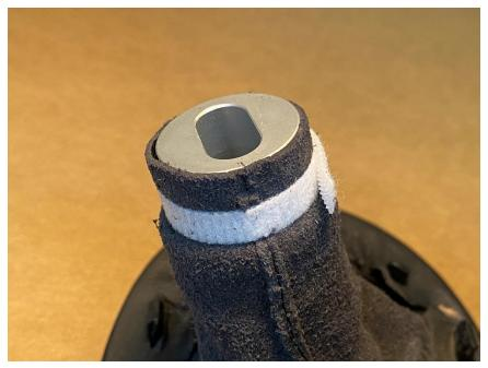
2. Pull the shaft up through the boot and pull the boot down past the bottom lip of the shaft so that it lays evenly and fully beneath the bottom lip.
