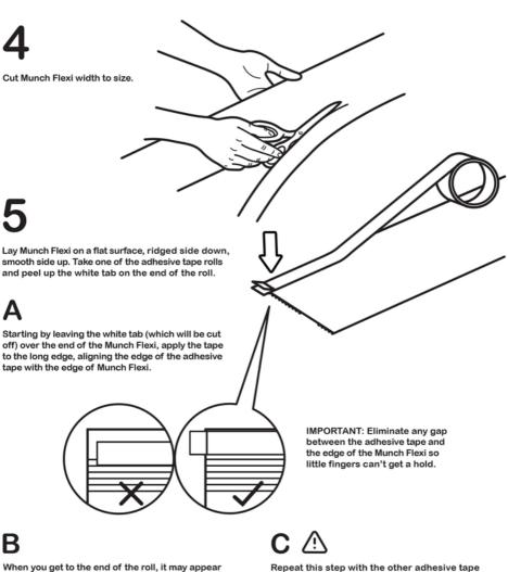
When you get to the end of the roll, it may appear that the adhesive tape is not long enough. However, peel the white liner completely off the roll core, then separate the white liner from the red liner, exposing the last section of the adhesive tape strip. Apply this to the Munch Flexi then trim the end.
