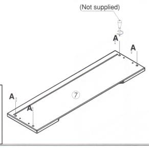
Step 2: Assemble Drawer Back Panel and Side Panels.
