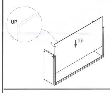
Step 4: Assemble Drawer Front Panel.
