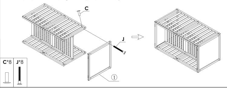
Stage 5: Connect the feet to the end panels & side panels with the 8\*H connecting bolts provided.
