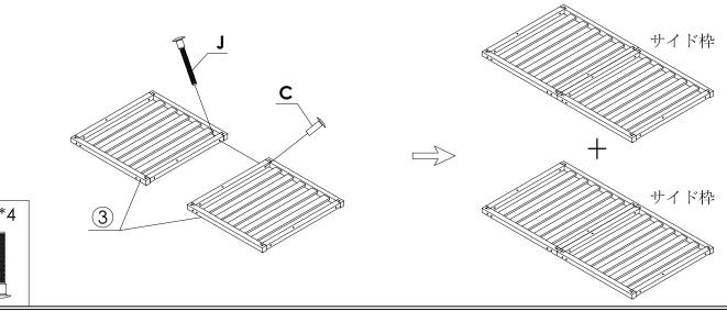
Stage 3: Connect two base panels and four side panels with the 4\*G+4\*I connecting bolts provided. GとIで床板をサイド枠に取り付けます。
