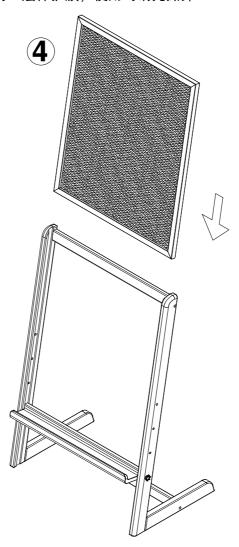
▲ Tighten all the connecting bolts. 锁紧所有螺丝。
