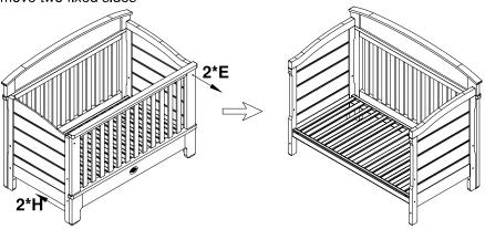
Stage 2: Block the top holes with the 2\*E connecting bolts and 2\*A capping nuts provided
