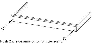
**Stage 3:** Fix to the back of chest with 2**x** B connecting bolts.
