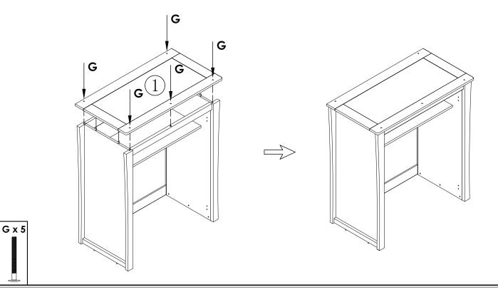
Step 6: Attach the Drawer Cabinet using 4 x G connecting bolts.
