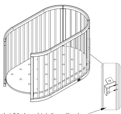
Install the base plate in the position shown.
