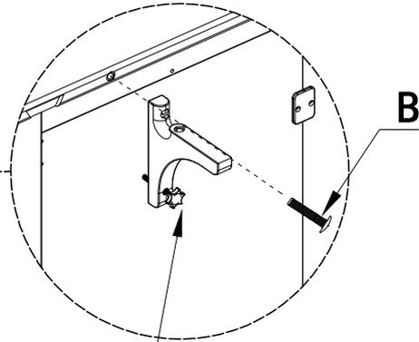
Adjust the star knob bolt so that it applies a bit of pressure to the backboard of the chest.
