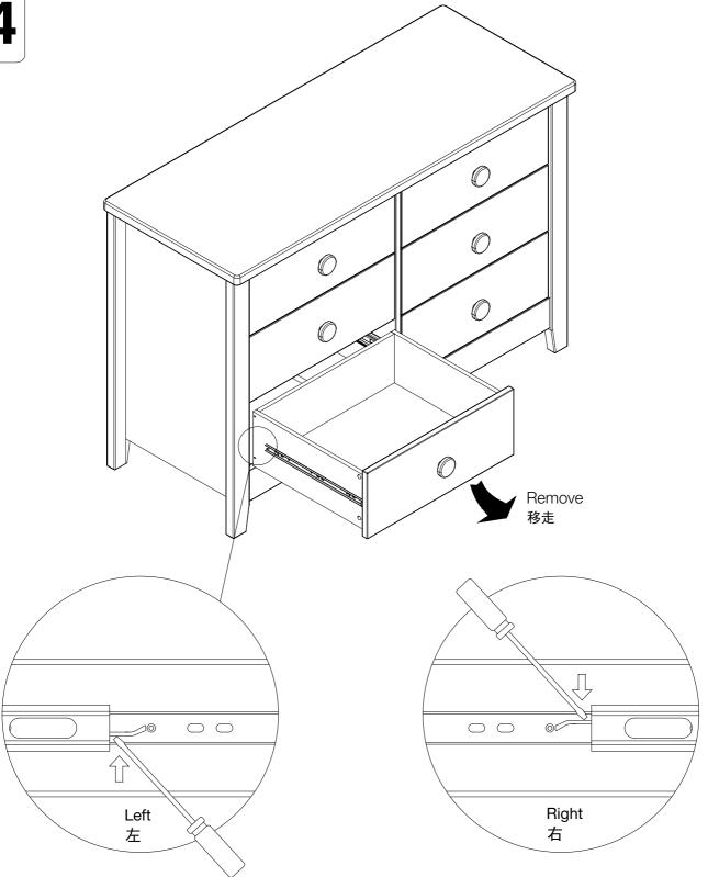
**Note:** 1. Insert a small screwdriver inside the Right Hand Side drawer runner. Push down the tip of the drawer locking mechanism.
