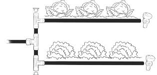
If you're installing rows of soaker hoses, space them 12 to 18 inches apart on sandy soil, or 18 to 24 inches apart on clay or loam soil. For small annuals, space rows of soaker hoses 12 to 18 inches apart regardless of soil type to ensure their roots receive sufficient water.
