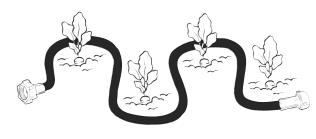
Stretch the soaker hose straight for crops or flowers planted in a straight line, or weave the hose in a nice flowing curve among plants spaced more randomly. Place the soaker hose about two inches from plant stems, or closer for new plantings or annuals, which tend to have less shallow roots. When installing, make every effort to keep the soaker hose as flat as possible to avoid uneven watering.
