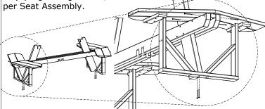
3. Set together both Leg Assemblies installing 4 - 2 1/2" Screws .
