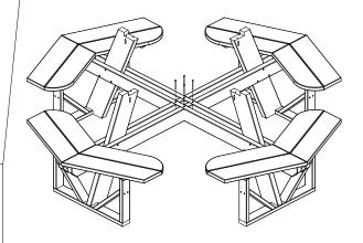
4. Attach (A) Top to assembled Base from step 3 using 8 - 2" Screws in Pocket Holes .
