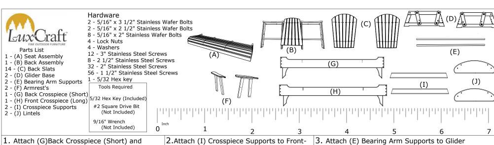
(H) Front Crosspiece (Long) to (D) Glider Base's Back Crosspieces using 4 - 2" Screws per Using 8 - 2" and 6 - 3" Screws per side, be sure to match all numbers & or letters.
