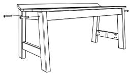
2. Attach (D) Cross Pc. to (B) & (C) Leg Assemblies using 2 1-1/2" Screws per side in predrilled holes.
