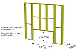
The plaster cutout dimensions are shown at right. Cutout size 1390mm wide and 785mm high 785mm 1390mm
