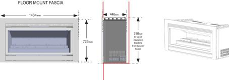
Please note: Realistic gas log fires can be installed as either wall mounted or floor mounted. The Flue system must be installed by an Authorised installer. Some installations may require the provision of a hearth to protect the floor from radiant heat. Contact your Illusion dealer for more information.
