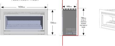
Please note: Realistic gas log fires can be installed as either wall mounted or floor mounted. The Flue system must be installed by an Authorised installer. Some installations may require the provision of a hearth to protect the floor from radiant heat. Contact your Illusion dealer for more information.
