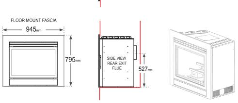
Please note: Matrix gas log fires fascias are available as either wall mounted or floor mounted. See above drawings for fascia sizes. The Flue system must be installed by an Authorised installer.
