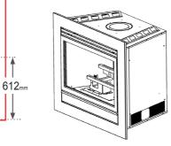
Please note: Matrix gas log fires fascias are available as either wall mounted or floor mounted. See above drawings for fascia sizes. The Flue system must be installed by an Authorised installer Some installations may require the provision of a hearth to protect the floor from radiant heat. Contact your Illusion dealer for more information.
