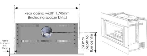
Please note: Luminar gas log fires can be installed as either wall mounted or floor mounted. The Flue system must be installed by an Authorised installer. Some installations may require the provision of a hearth to protect the floor from radiant heat. Contact your Illusion dealer for more information.
