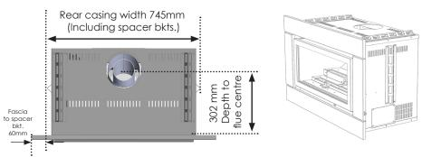
Please note: Azura gas log fires can be installed as either wall mounted or floor mounted. The Flue system must be installed by an Authorised installer. Some installations may require the provision of a hearth to protect the floor from radiant heat. Contact your Illusion dealer for more information.
