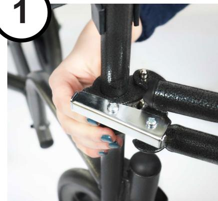
**EN** 1. **To remove the footrests**, use the metal lever to unclip the footrests and remove them from the chair frame.
