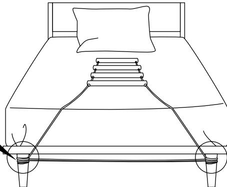
**EN** Tie the rope to the legs of the bed forming several circles around the leg until it is securely fastened. The height of the ladder will depend on the number of turns around the legs.
