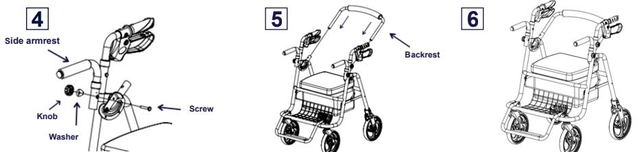
3. Finally, put the backrest tube (B) into main frame (A) push button until you hear "Click".
