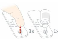
**Avoid trapping air bubbles in the specimen well (S) and do not add any solution to the result area.**
