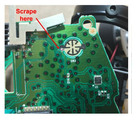
Solder wire to newly exposed copper. This wire should be around 2.25 inches (55mm) long.
