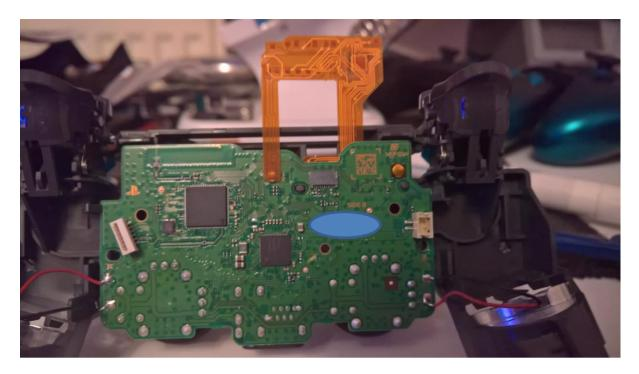
You can add some hot glue to keep the mod chip down only add it where it blank see step 5 picture to see where to line the mod chip
