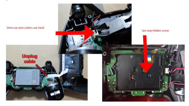
Step 3: Remove the circuit board.
