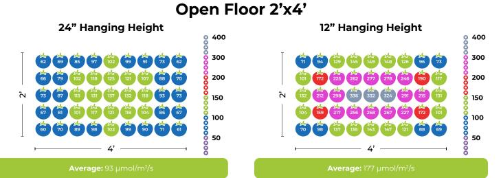
PPFD readings were taken using Active Grow 25W T5 HO Ballast Bypass 4FT LED Horticultural Lamps in Sun White Spectrum and an Apogee Extended Range PFD Sensor. Test results do not include reflective surfaces or adjacent lights.
