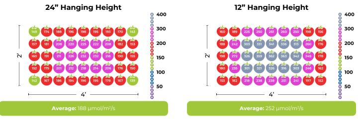
PPFD readings were taken in an Active Grow Walden Tent 2'x4' using Active Grow 25W T5 HO Ballast Bypass 4FT LED Horticultural Lamps in Sun White Spectrum and an Apogee Extended Range PFD Sensor.
