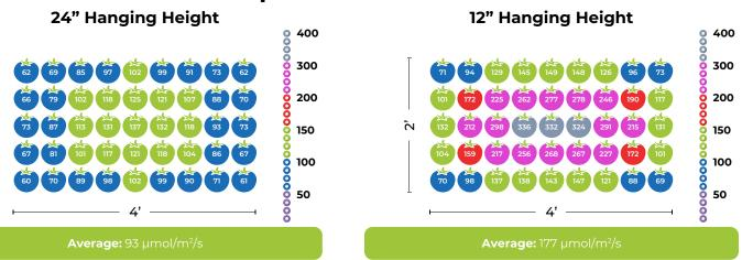
PPFD readings were taken using Active Grow 25W T5 HO Ballast Bypass 4FT LED Grow Lamps in Sun White Spectrum and an Apogee Extended Range PFD Sensor. Test results do not include reflective surfaces or adjacent lights.
