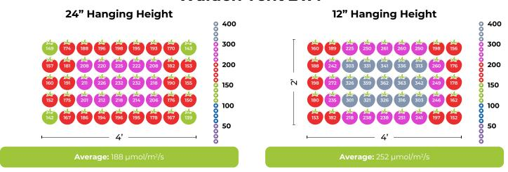
PPFD readings were taken in an Active Grow Walden Tent 2'x4' using Active Grow 25W T5 HO Ballast Bypass 4FT LED Grow Lamps in Sun White Spectrum and an Apogee Extended Range PFD Sensor.
