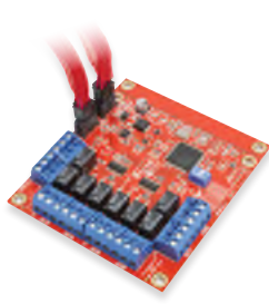
996515PCB&K Integrati UniBus 8 Relay Auxiliary Expander PCB & Accessories (Includes 270mm UniBus patch cable)
