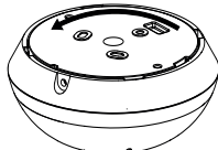
Figure 2. Removing the bracket
